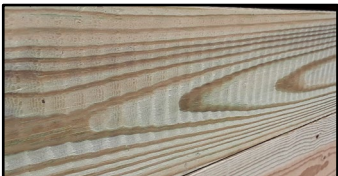
Wavy dressing due to loose holding devices, poor cutting circle, dull knives, and other causes
