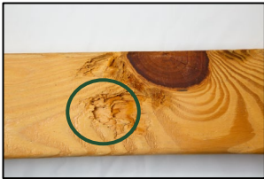
Torn grain due to tearing of fiber by knives or saws
