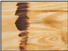
Machine burn due to piece sticking in planer
