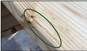
Improper eased edge adjustment
