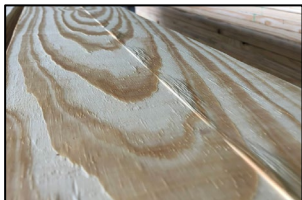
Knife gap due to damaged planer knife or knives
